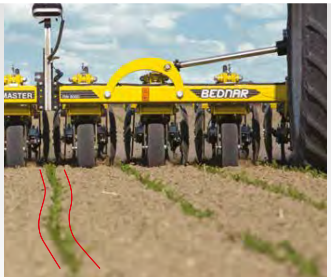
The self-guidance system is able to guide a Row-Master even if crops are seeded in an arc.
