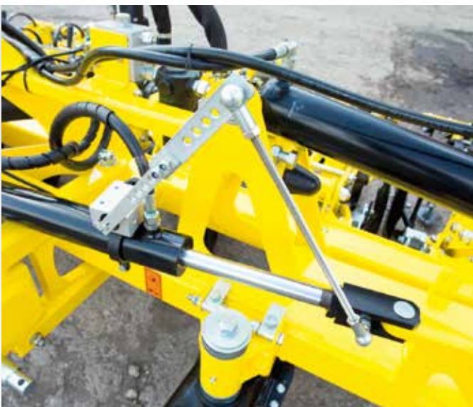
Sensor of the current position of the machine frame in relation to the 3-point hitch.
