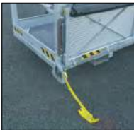
2 roof presence sensors
