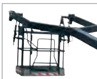
Pendular platform allows work under-bridges
