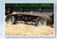
HAWE offers a wide selection of low-compaction tyres up to 1.70 m diameter and also caterpillar drives for the increased mobility and off-road capability of our transfer trailers.
