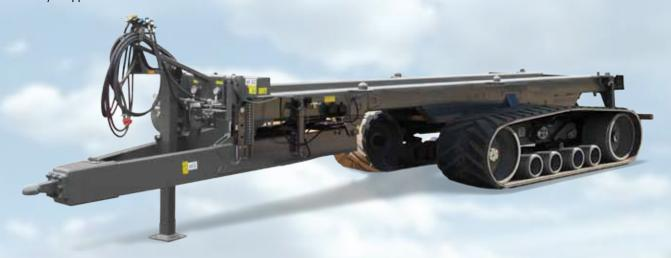
As another ground-friendly suspension concept we offer with the TERRA TRAC tracks an axle bridge driven by oil motors. The combination of high road speeds and high mobility in the field with high payload convinces the users. With the continuous development of this concept, the advantages of this chassis concept will be further expanded and used for a much wider range of applications.
